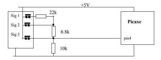
When signal 1 is high the voltage on pin4 is 0.25 \* 5V = 1.25VWhen signal 2 is high. The voltage on pin4 is 0.6 \*5V=3.0V
