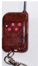
As a first example of a program, I use simple 'keyfob' type radio controllers. These have 4 outputs of which I use 3 – A for accelerate, B for Brake and D for toggle direction. The outputs are normally low and go to +5V when the transmitter button is pressed. So we just need a program to check the button state and adjust the motor speed and direction accordingly. So I use pin1 for 'A', pin3 for 'B' and pin4 for 'D" in the circuit above.
