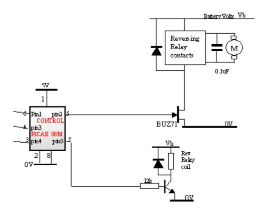
The Picaxe programming will depend on what kind of radio control you have – the circuit above just shows there are 3 available inputs to get the info into the Picaxe. eg accelerate, brake and toggle direction. all you need to do is decide in the program what to do and use the PWMOUT command. It runs in the background, so the program can go and check the state of the input signals while the motor speed remain constant.
